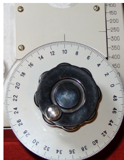
Fig. 3. Variable capacitor with a resolution of 0.2 pF and a capacitance range from 50 to 1150 pF
